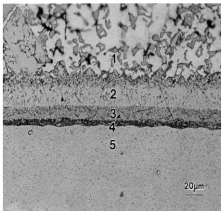
Fig. 2. Picture of the soldered intermetallic layers on a H13 pin.
