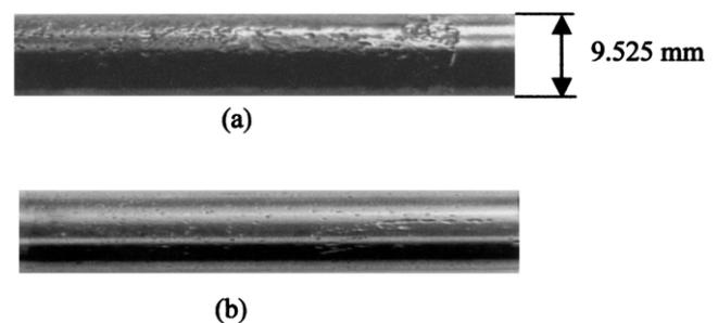
Fig. 8. (a) Uncoated H-13 pin after 2 h at 680°C in molten aluminum A380.1. (b) Ti/TiN coated pin after 2 h at 680°C in molten aluminum A380.1.
