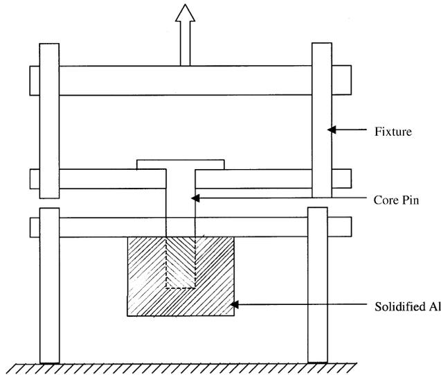
Fig. 4. Schematic of the ejection test set up.
