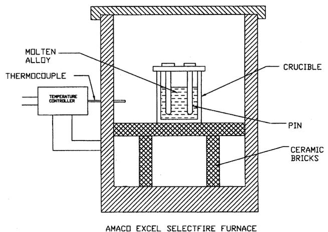
Fig. 3. Schematic illustration of the accelerated corrosion test setup at the Ohio State University.
