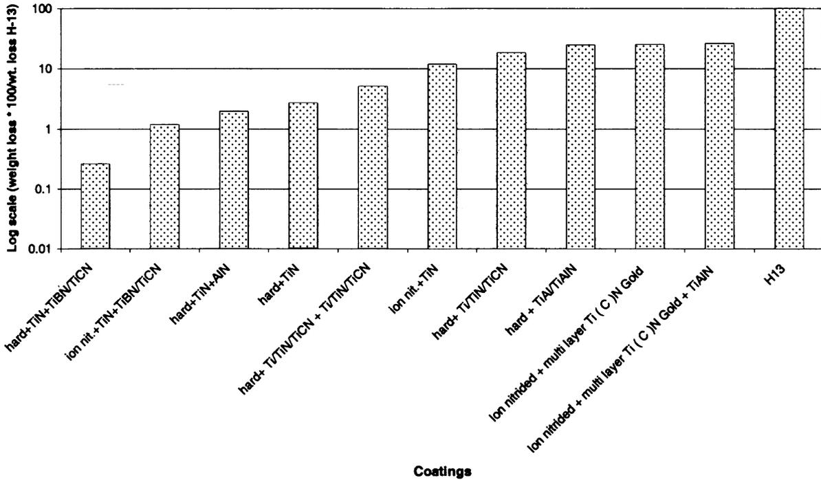
Fig. 5. The performance of all the LAFAD coating candidates as compared to H-13. The weight loss per unit area is represented on a log scale and normalized to 100 for H-13 [7].
