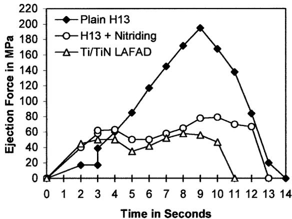
Fig. 7. The change in a force during ejection for the three surface treated coupons uncoated, nitrided and multilayer coated.
