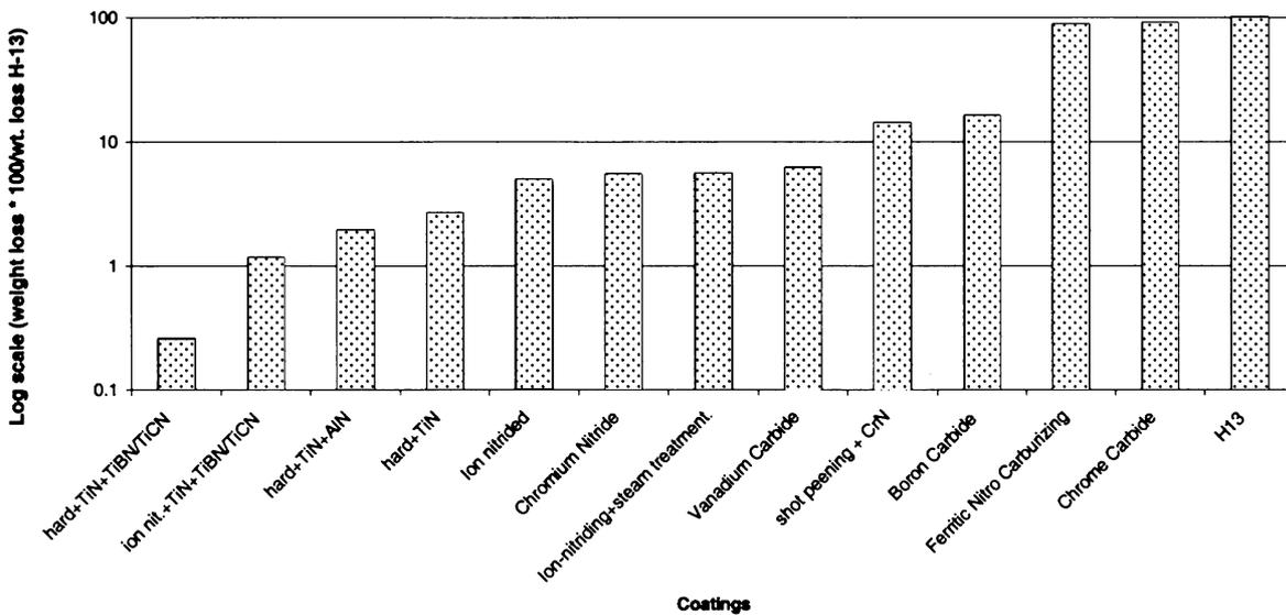
Fig. 6. Performance of the LAFAD multilayer coatings as compared to other coatings testes previously at the Ohio State University. This graph has been normalized by assigning a value of 100 to H-13. Weight loss per unit area is represented on a log scale [7].
