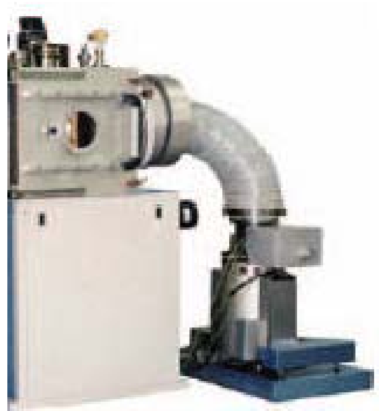
Quarter-torus tubular solenoid- plasma duct
