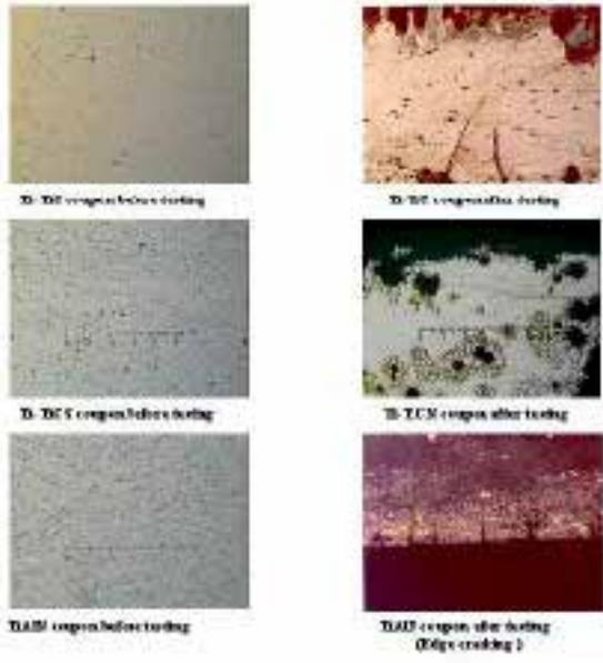
**Figure 7** – Surface characteristics of multilayer Ti/TiC, Ti/TiCN and Ti/TiAlN coated coupons before and after thermal cycling for 1000 cycles.
