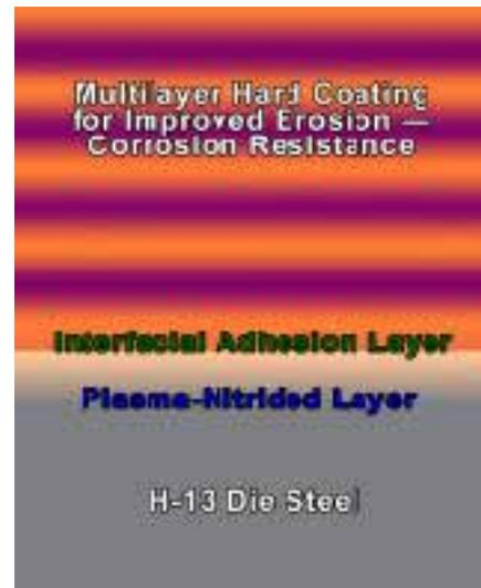
Figure 2 – Schematic of multilayer coating system.
