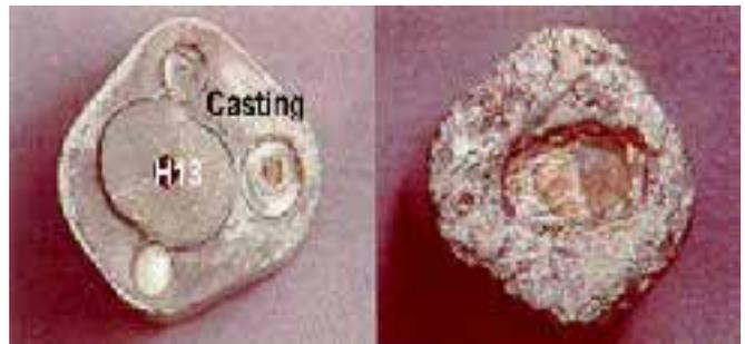
Figure 1 – Picture of a soldered pin.
