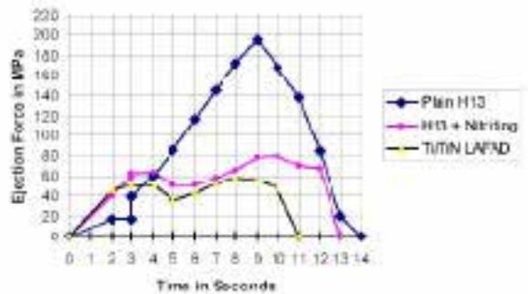
**Figure 6** – The change in a force during ejection for the three surface treated coupons uncoated, nitrided and multilayer coated.
