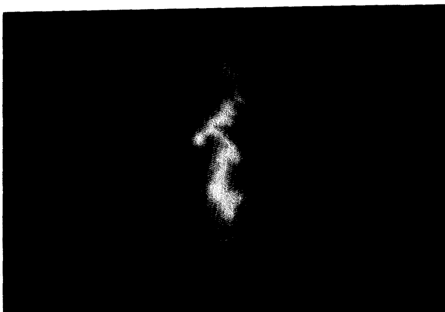
Fig. 3. The linear vacuum electric arc evaporator with titanium cathode of area 100 \times 400 \text{ mm}^2 , I_c = 350 \text{ A} . A luminescent trace of the vacuum arc cathode spots is visible.
