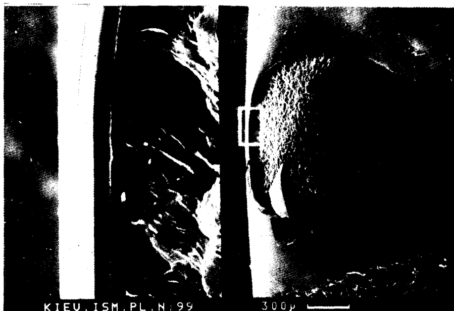
Fig. 10. A stretch of i-C coating on melted aluminium surface.
