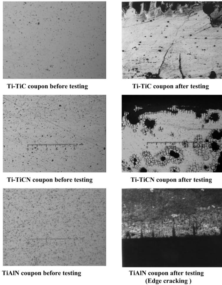
Fig. 8. Coupons with different coatings before and after testing 1000 cycles at 50× magnification.
