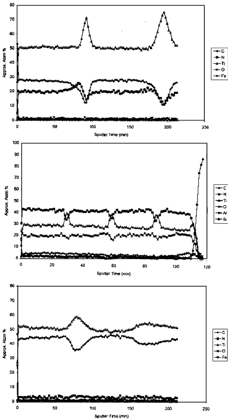
Fig. 2. AES depth profile analysis of Ti/TiCN, Ti/TiAlN and Ti/TiC coatings.
