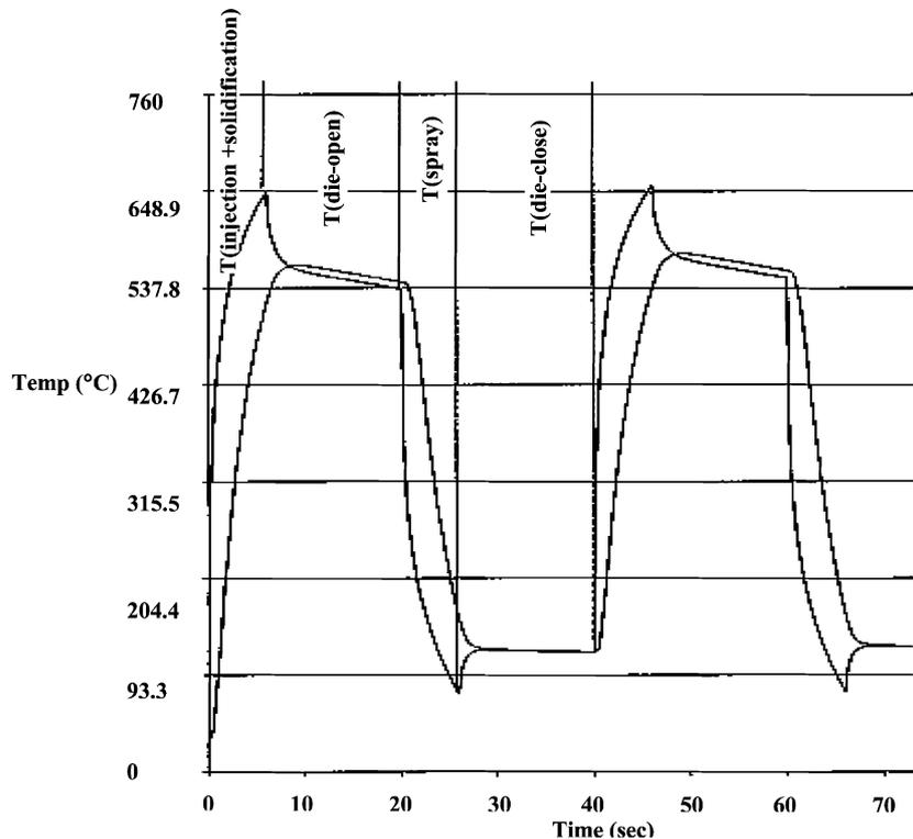
Fig. 3. The time–temperature plot obtained from the DEFORM simulations.
