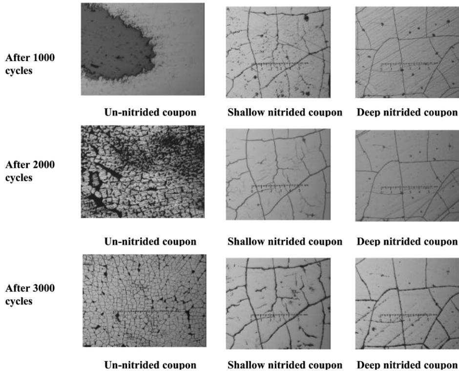
Fig. 5. Results of testing of nitrided H-13 coupons at 50× magnification.
