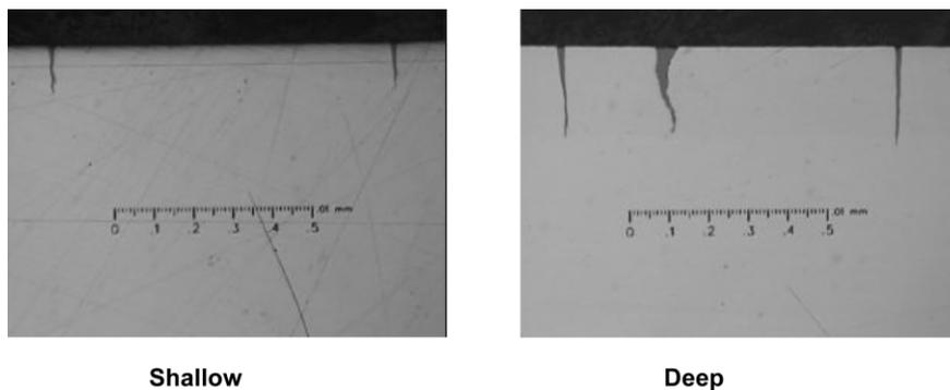
Fig. 6. Micrograph of cracks inside shallow and deep nitrided H-13 coupon after 3000 cycles (100×).
