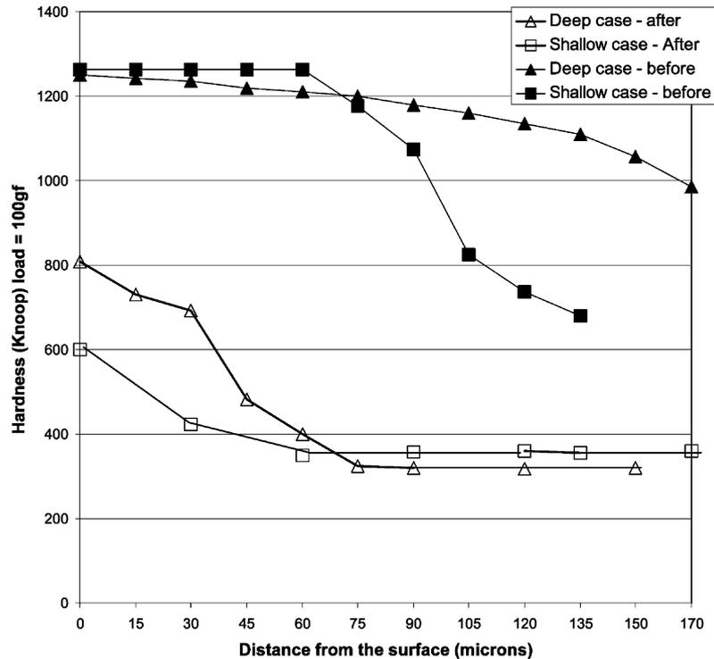
Fig. 7. Microhardness profiles of nitrided samples before and after testing (3000 cycles).
