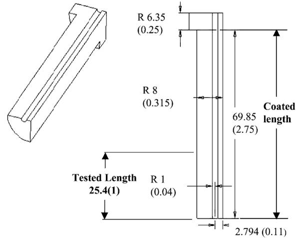
Fig. 4. Test coupon. All dimensions in mm. Dimension in parenthesis are in English units.
