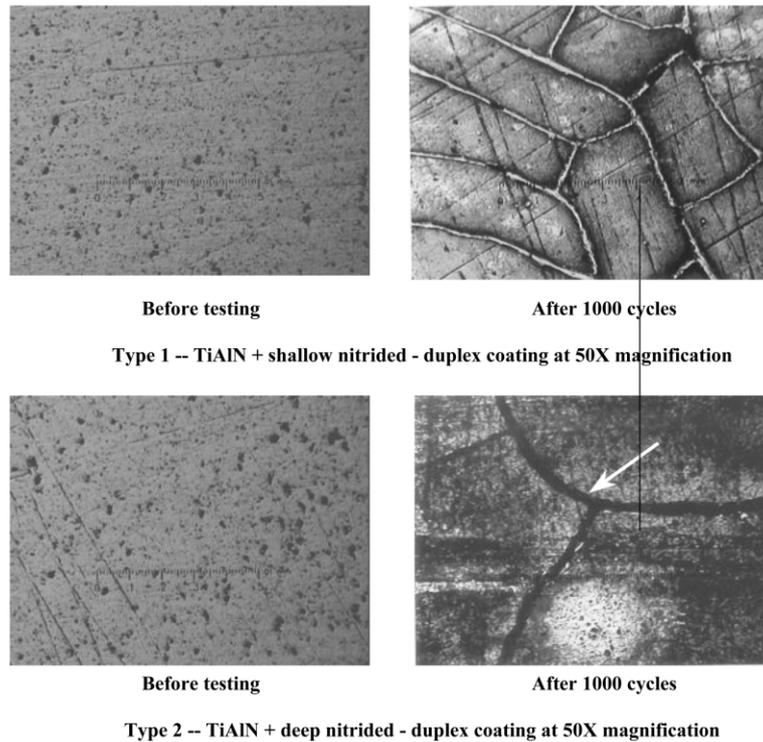
Fig. 9. Result of duplex coating system.
